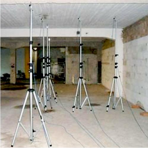
Digital instrumentation for deflection measurement of structures, 58-C0239/A complete system with 3 additional measurement elements (58-C0239/A1 q.ty 3)
